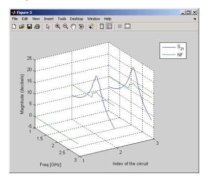
The budget plot shows parameters as a function of frequency by circuit index. Components are indexed based on their position in the network. In this example:
