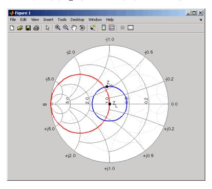
**6 Find the intersection points.** After you draw the input SWR and constant conductance circles, you can find the points of intersection that correspond to the two possible solutions. Because only one solution is necessary, choose the lower-half intersection point, and designate this as the solution point A. Use the following code to plot and label this intersection point on the Smith chart using the reflection coefficient calculated from the admittance value:
