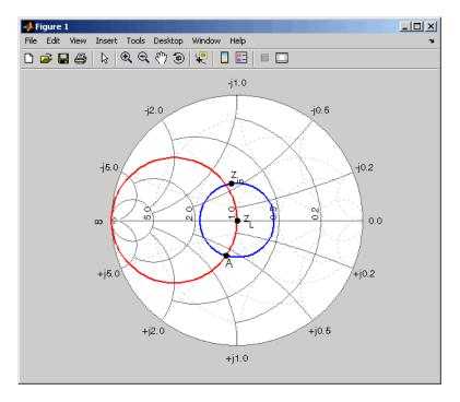
**7 Calculate the required lengths.** Based on the intersection point A, you can find the required lengths of the series transmission line and
