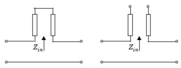
$\boldsymbol{Z}_{in}$  is the input impedance of the series circuit. The ABCD-parameters for the series stub are calculated as
