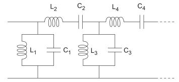
Where  $[L_1,L_2,L_3,L_4,...]$  is the value of the 'L' property, and  $[C_1,C_2,C_3,C_4,...]$  is the value of the 'C' property.
