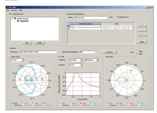
**4** Select or deselect the S-parameter check boxes at the bottom of each plot to customize the parameters that the plot displays. Use the pull-downs at the top of each plot to customize the plot options.
