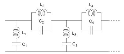
Where  $[L_1,L_2,L_3,L_4,...]$  is the value of the 'L' property, and  $[C_1,C_2,C_3,C_4,...]$  is the value of the 'C' property.
