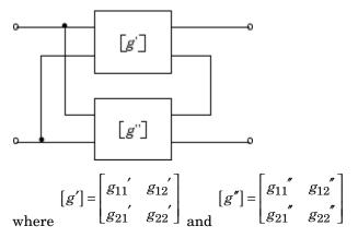
The analyze function then calculates the g matrix for the inverse hybrid network by calculating the sum of the g matrices of the individual networks. The following equation illustrates the calculations for two 2-port networks.
