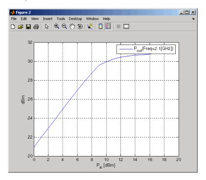
**Note** The plot shows the power data at 2.1 GHz because this frequency is the one for which power data is specified in the default.amp file.
