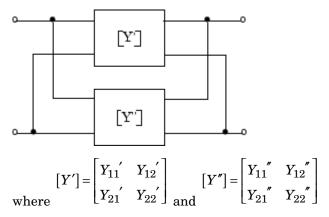
The analyze function then calculates the admittance matrix for the parallel network by calculating the sum of the individual admittances. The following equation illustrates the calculations for two 2-port circuits.
