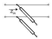
$\mathbf{Z}_{in}$  is the input impedance of the shunt circuit. The ABCD-parameters for the shunt stub are calculated as
