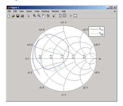
**Note** The plot shows the S-parameters over the frequency range for which network data is specified in the default.amp file — from 1 GHz to 2.9 GHz.
