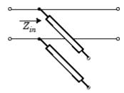
$Z_{\it in}$  is the input impedance of the shunt circuit. The ABCD-parameters for the shunt stub are calculated as
