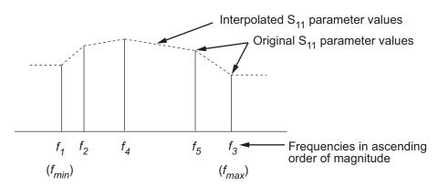
You can specify the interpolation method as Cubic, Linear (default), or Spline. For more information, see "One-Dimensional Interpolation" and the interp1 reference page in the MATLAB documentation.
