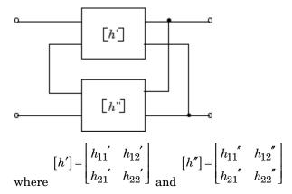
The analyze function then calculates the h matrix for the hybrid network by calculating the sum of the h matrices of the individual networks. The following equation illustrates the calculations for two 2-port networks.
