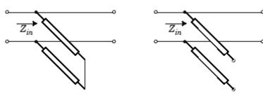
$Z_{\it in}$  is the input impedance of the shunt circuit. The ABCD-parameters for the shunt stub are calculated as
