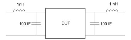
In this example, you remove the effects of the fixture and extract the S-parameters of the DUT.
