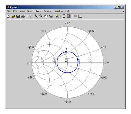
**5 Draw the constant conductance circle.** To find the required susceptance to move the 50-ohm load admittance to the SWR circle, you must define the constant conductance circle. To define the circle, you
