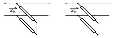
$\mathbf{Z}_{in}$  is the input impedance of the shunt circuit. The ABCD-parameters for the shunt stub are calculated as
