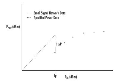
If  $\Delta P$  is more than 0.4 dB, a warning appears. Large discrepancies may indicate measurement errors that require resolution.
