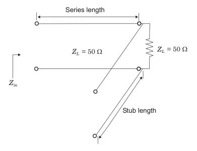
You begin by finding the required transmission line lengths for the single-stub matching networks. Then, you cascade the matching networks with the amplifier and visualize the results.
