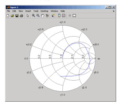
4 View the 75-ohm S-parameters and Y-parameters at 6 GHz. Type the following set of commands at the MATLAB prompt to display the four 75-ohm S-parameter values and the four Y-parameter values at 6 GHz.
