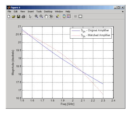
You can compare the matched amplifier results with the expected transducer gain (in dB). From the S21 parameters plot, you can see that the gain of the matched amplifier at 1.9 GHz is between 19 dB and 19.5 dB. The expected gain is given by the following equation:
