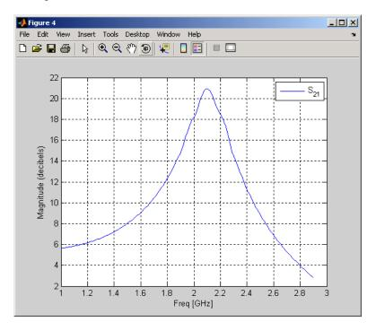
**3** Type the following set of commands at the MATLAB prompt to use the plot command to create a budget plot of the S21 parameter and the noise figure of the amplifier network:
