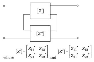
The analyze function then calculates the impedance matrix for the series network by calculating the sum of the individual impedances. The following equation illustrates the calculations for two 2-port circuits.
