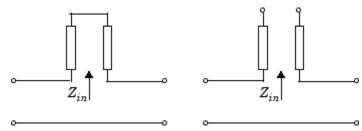
$Z_{\it in}$  is the input impedance of the series circuit. The ABCD-parameters for the series stub are calculated as
